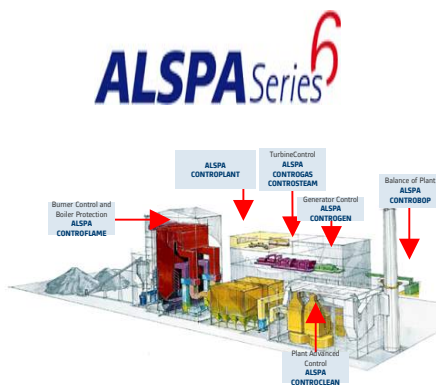
New Automation System suite
